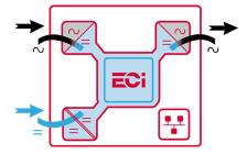
From **1 to 4 modules**, with several **options** available (manual external by-pass and AC distribution), the Bravo 6 modular inverter is also **hot-swappable** meaning a very easy and cheap maintenance. The modules are delivered with our new monitoring solution.
